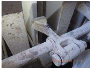
Picture 50: CE hammer still in good condition
