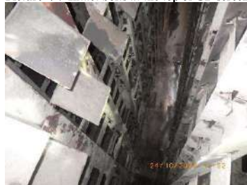
Picture 9 : Intact inlet guide vane
