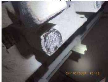
Picture 32: Slightly worn-out anvil
