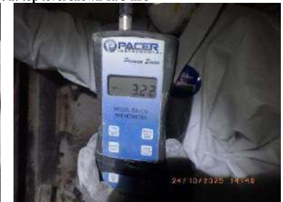
Picture 75 and 76: GD test at top level shown 3.22 m/s
