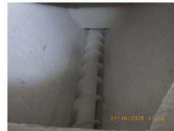
Picture 20: Screw conveyor still in good condition
