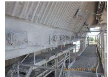
Picture 21: Hopper heater was intact
