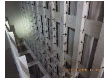
Picture 13: Normal GD screen condition
