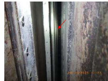
Picture 53: Slightly bent DE
