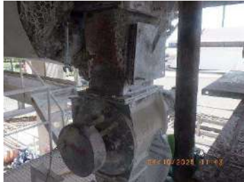
Picture 23: Balance line flange not completely close
