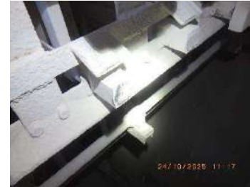
Picture 51: Rapping bar spacer still in good condition
