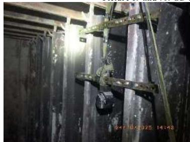
Picture 71 and 72: GD test at top level shown 0.56 m/s
