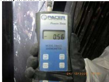
Picture 71 and 72: GD test at top level shown 0.56 m/s
