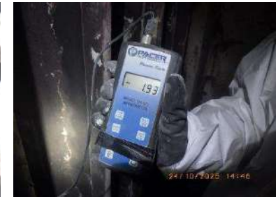
Picture 73 and 74: GD test at top level shown 1.93 m/s
