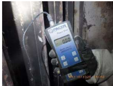
Picture 69 and 70: GD test at top level shown 0 m/s
