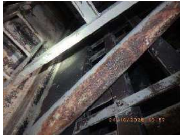
Picture 10 : Intact side baffle plate of GD screen
