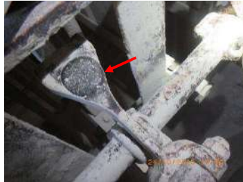
Picture 29: Slightly worn-out on CE hammer
