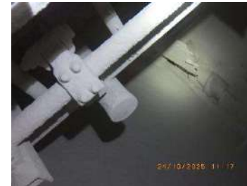
Picture 60: DE anvil still tolerable condition
