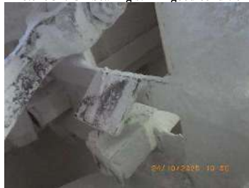
Picture 33: Rapping bar spacer still in good condition
